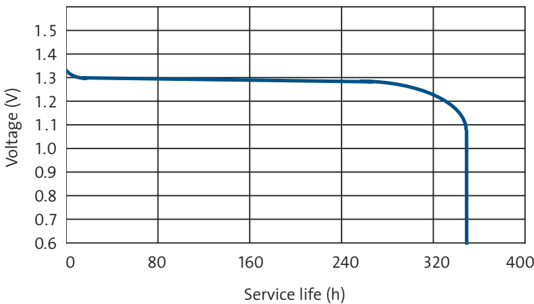
Discharge characteristics at 1.500 Ω, 25°C and 60 % Relative Humidity (Discharged 24 hours/day)
