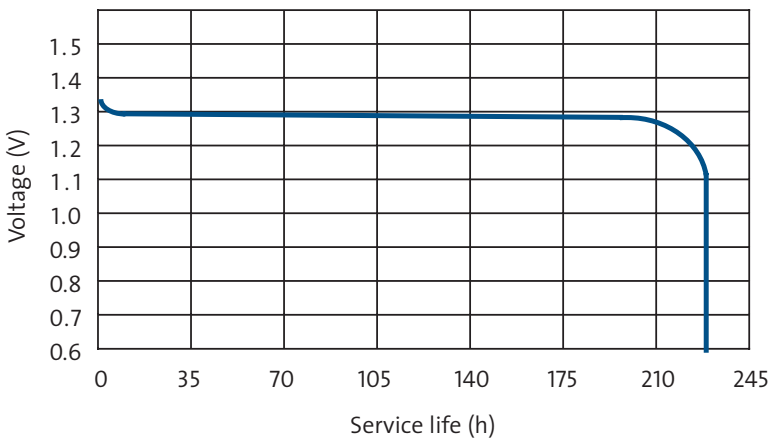
Discharge characteristics at 3.000 Ω, 25°C and 60 % Relative Humidity (Discharged 24 hours/day)
